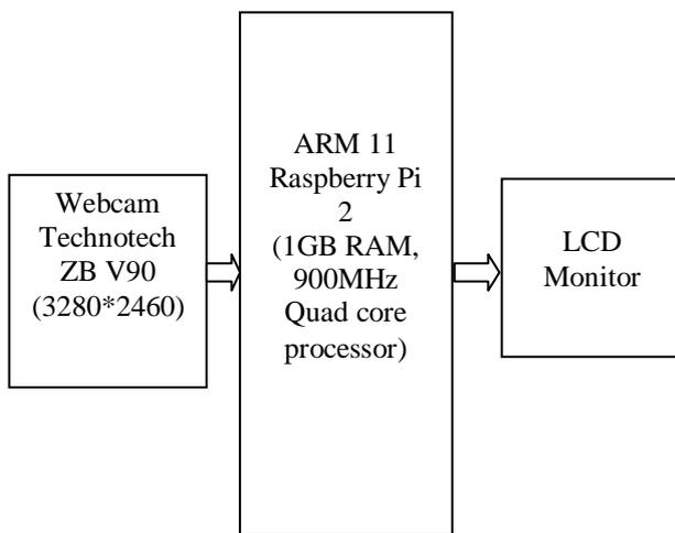
Fig. 1 Overview of System Architecture
